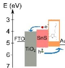
*Band diagram of investigated SnS NC based solar cells*
