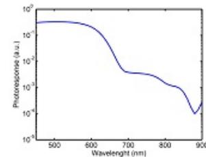
*Spectral response showing sensitization of polymer-based solar cells in the NIR due to incorporation of SnS NCs*
