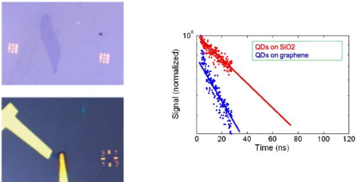
**Figure 2: (left) Contacted graphene flakes. (right) Emission lifetime of PbS quantum dots on graphene and silicon**
