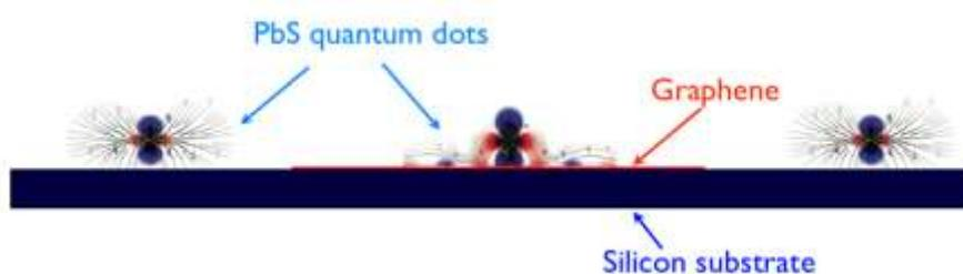
**Figure 1: schematic representation of energy transfer from emitters to graphene. The gray lines represent the Poynting vectors. Strong energy transfer to graphene is expected due to the unique properties of graphene.**
